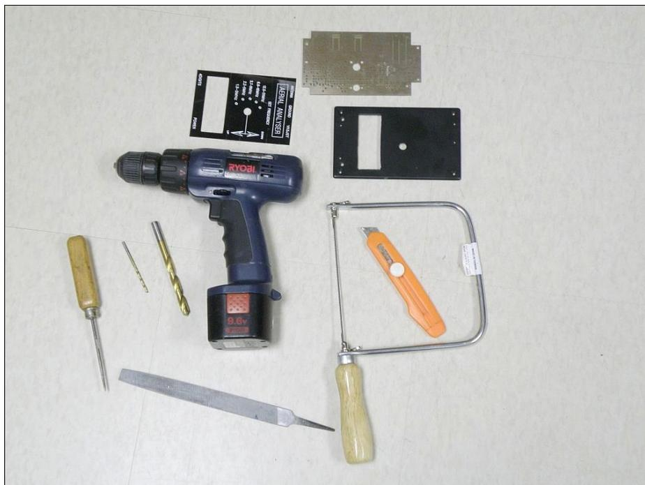
The bare circuit board serves as a template for drilling the frequency rotary switch (center) and the board mounting holes (2 at each end). The mounting holes used by the binding posts (left end) will be made bigger later. There is no template for drilling the switch holes (right end at top and bottom), but now is a good time to locate two places for the switches and drill their holes.
