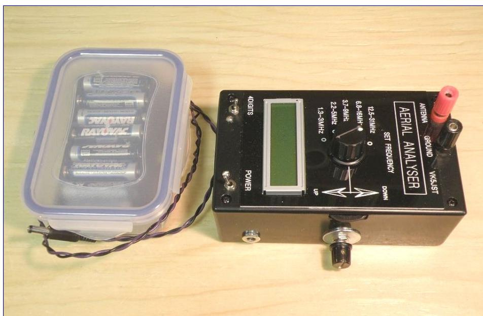
To transport my VK5JST Aerial Analyser and carry it into the field I made a case out of a plastic CD box from Wal-Mart. There is a removable shelf with a wood handle. The battery pack and other bits and pieces are stored under the shelf.
