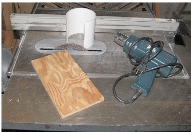
Picture 2. Making the Variable Capacitor Shield
