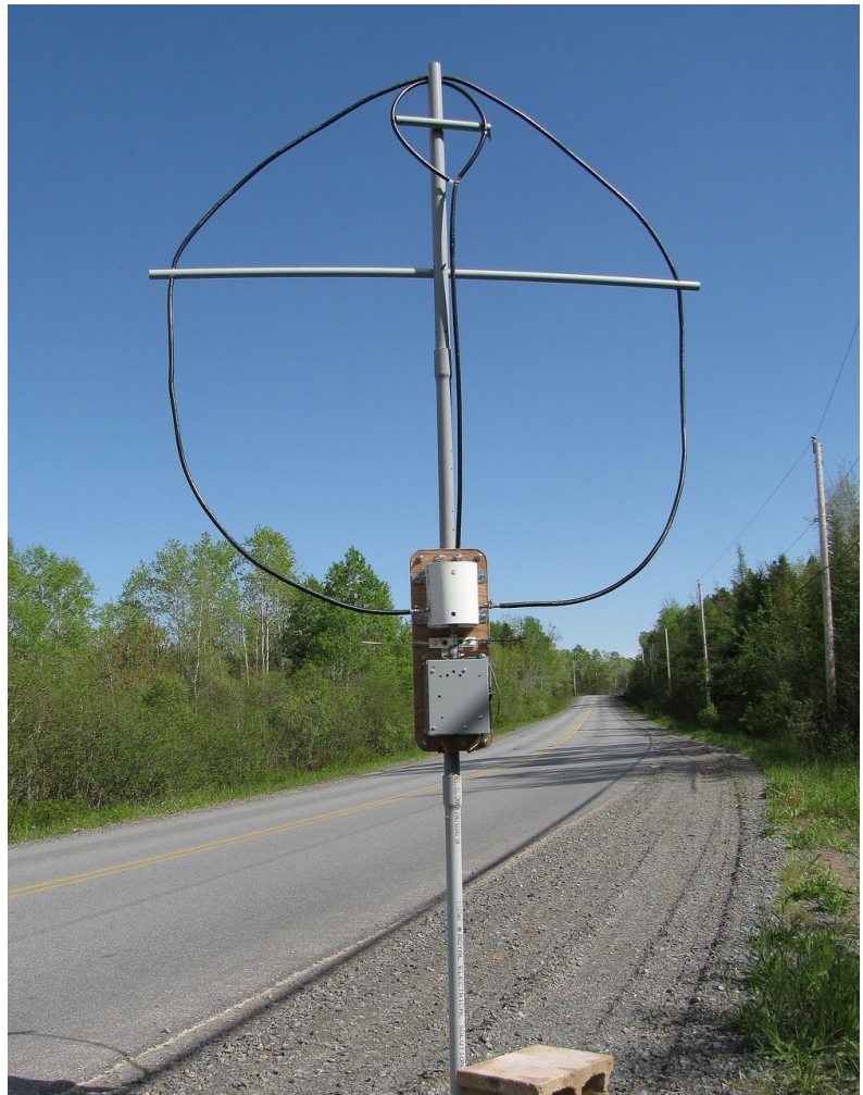
Picture 8. Autotuner Mounted on Mast of Small Magnetic Loop Antenna
